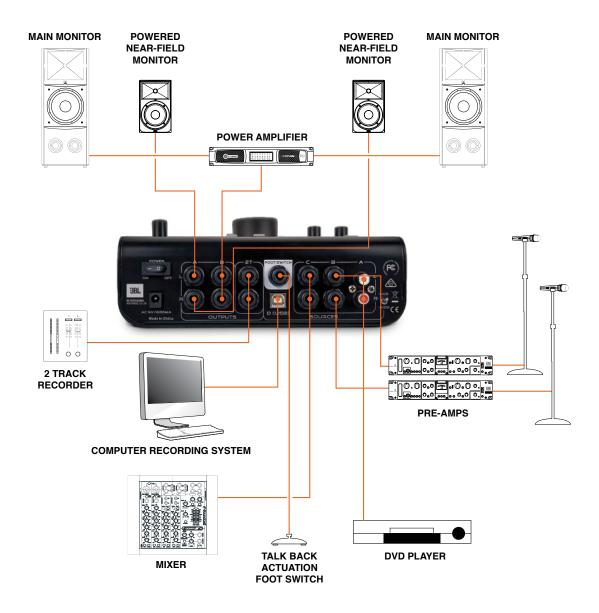
When connecting PASSIVE speakers, you must first connect the output of the ACTIVE-1 to a power amplifier and then connect the amplifier to the speakers.
