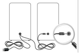
The headphone port can be used to connect a wired headphone. As soon as the headphone is connected, the speakers will be muted. The volume knob controls level for both speaker & headphone out.
