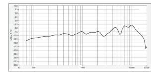
FREQUENCY RESPONSE CURVE CSDM04 USB POWERED SPEAKERS
